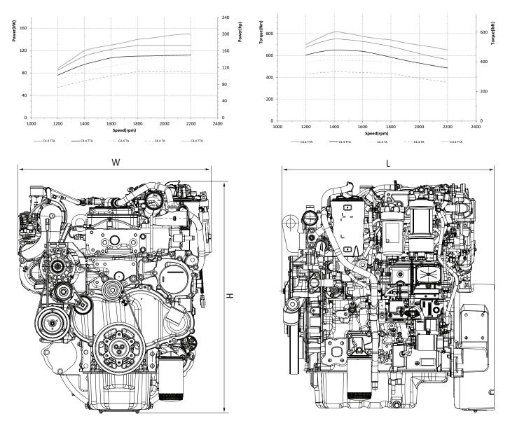
The above dimensional drawings are based on the twin turbocharged aftercooled model
